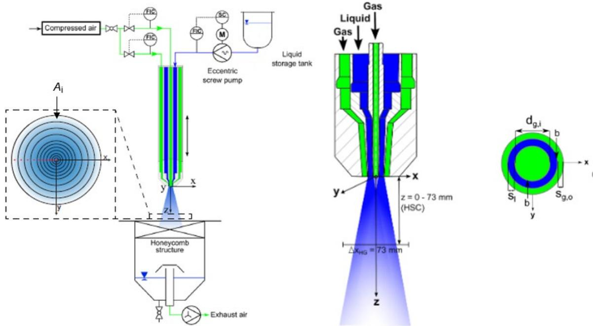
**Figure 1.** Schematic of the experimental setup (left). Scheme (middle) and top view of the nozzle (right).
