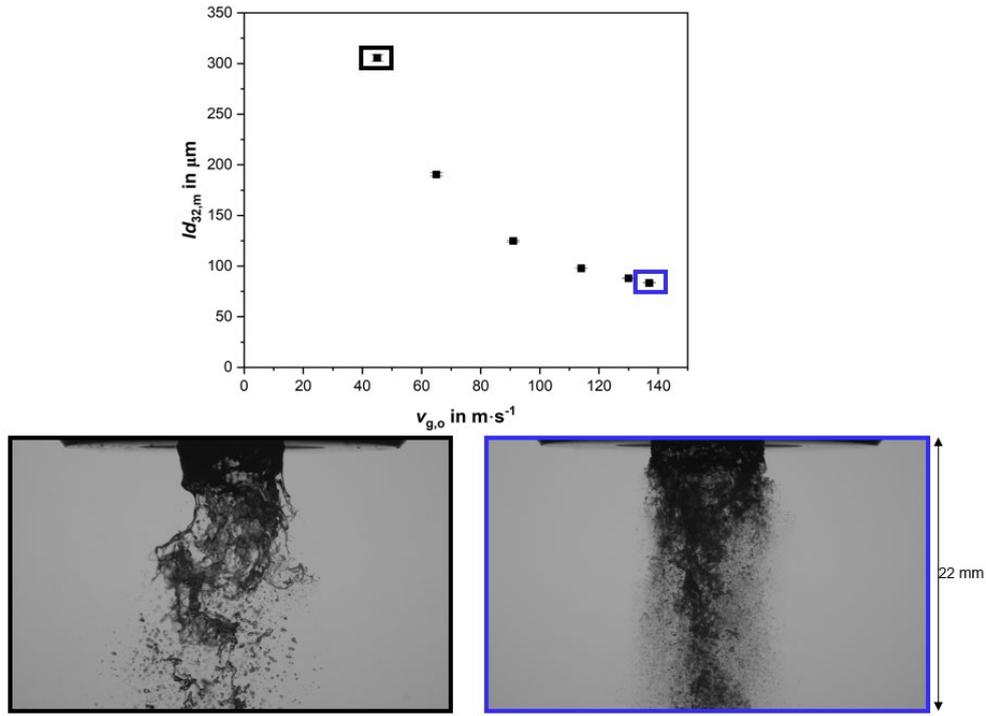
**Figure 3.** Top: Mass-weighted integral Sauter mean diameter ( $Id_{32,m}$ ) at  $z = 300$  mm below the nozzle orifice as a function of outer gas velocity ( $v_{g,o}$ ). Bottom: HSC images of primary sheet breakup;  $v_{g,o} = 46 \text{ m}\cdot\text{s}^{-1}$  (left);  $v_{g,o} = 137 \text{ m}\cdot\text{s}^{-1}$  (right). For all cases:  $v_{g,i} = 65 \text{ m}\cdot\text{s}^{-1}$ ,  $\dot{M}_l = 60 \text{ kg}\cdot\text{h}^{-1}$ ,  $\eta_l = 1 \text{ mPa}\cdot\text{s}$ .
