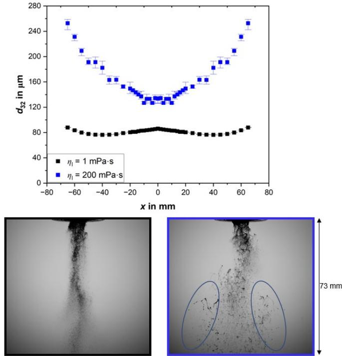
**Figure 2.** Top: Radial distribution of Sauter mean diameter ( $d_{32}$ ) at  $z = 300 \text{ mm}$  below the nozzle orifice as a function of liquid viscosity ( $\eta_l$ ). Bottom: HSC images of primary sheet breakup;  $\eta_l = 1 \text{ mPa}\cdot\text{s}$  (left);  $\eta_l = 200 \text{ mPa}\cdot\text{s}$  (right). For all cases:  $v_{g,i} = 65 \text{ m}\cdot\text{s}^{-1}$ ,  $v_{g,o} = 130 \text{ m}\cdot\text{s}^{-1}$ ,  $\dot{M}_l = 60 \text{ kg}\cdot\text{h}^{-1}$ .
