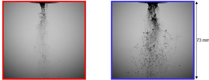
**Figure 4.** Top: Mass-weighted integral Sauter mean diameter ( $Id_{32,m}$ ) at  $z = 300$  mm below the nozzle orifice as a function of liquid mass flow rate ( $\dot{M}_l$ ) for varying liquid viscosities ( $\eta_l$ ). Bottom: HSC images of primary sheet breakup at  $\eta_l = 200$  mPa·s, for  $\dot{M}_l = 25$  kg·h<sup>-1</sup> (left) and  $\dot{M}_l = 93$  kg·h<sup>-1</sup> (right). For all cases:  $v_{g,i} = 65$  m·s<sup>-1</sup>,  $v_{g,o} = 130$  m·s<sup>-1</sup>.
