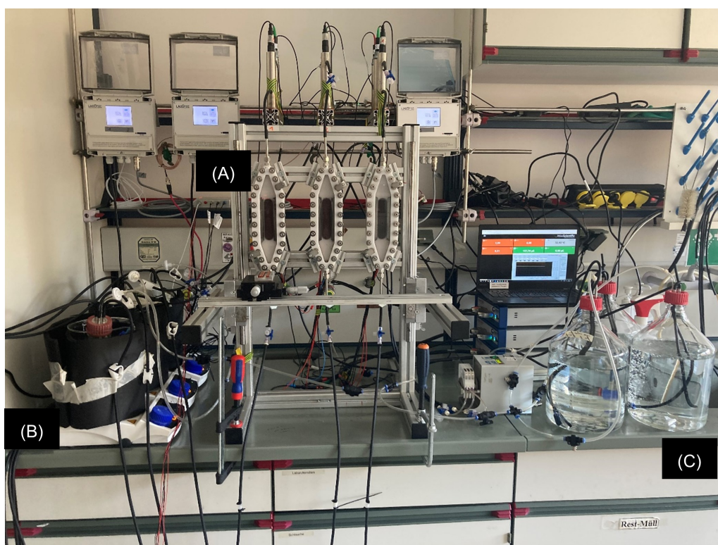
Figure 5.1: Experimental setup showing three flow cells (A) with integrated biofilm sensor operated in parallel. The cultivation medium was stored in flasks (B) and pumped with magnetic gear pumps (not in image) through the flow cells from bottom to top. Medium for the continuous operation was added into the piping system via peristaltic pump from storage flasks (C).
