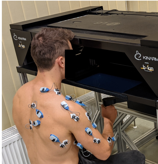
Figure 3.1: Experimental setup. A participant with EMG electrodes attached sits at the KINARM End-Point Lab (KINARM, Kingston, Canada).
