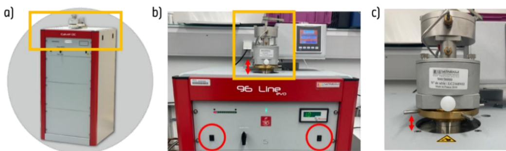
Figure 20. Optimization of the height, (a) overview of MHTC, (b) the upper part of the calorimeter with a focus on the sensor area and (c) how the height of the drop sensor can be adjusted by altering the height of the red height indicator arrow.
