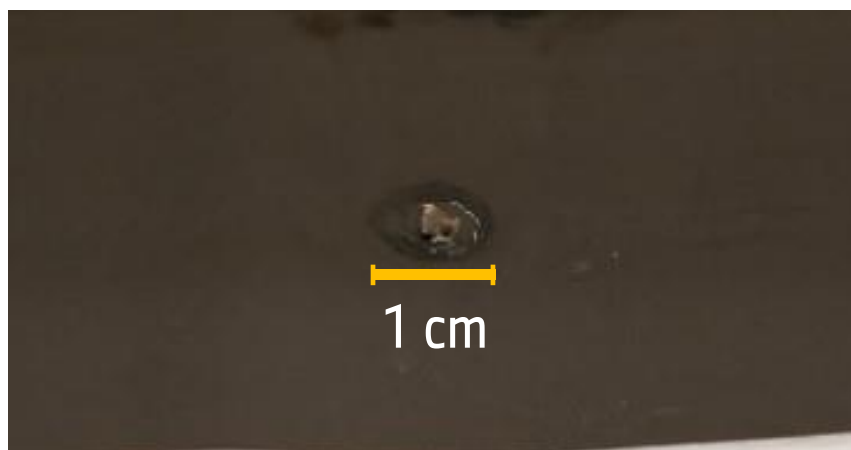
Figure 38. Post-test internal short circuit traces observed in a cell after nail penetration test.
