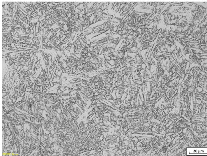
Figure 4.10 Microstructure including bainite and martensite in the HAZ close to the weld (Magnification 500x).
