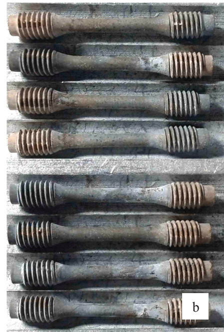
Figure 3. Appearance of EUROFER97-3 tensile specimens before (a) and after irradiation at 540 °C (b)
