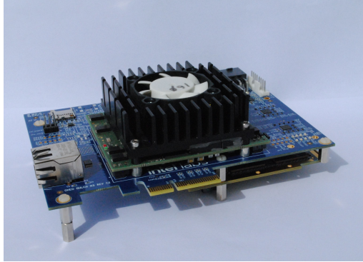
Figure 2.13.: The Kapoho Point system, featuring an Intel Loihi 2 chip on the Mezzanine Card (bottom), which is connected to an Intel Arria 10 FPGA SoM (top) via the Oheo Gulch Baseboard (middle). Figure adapted from [1].
