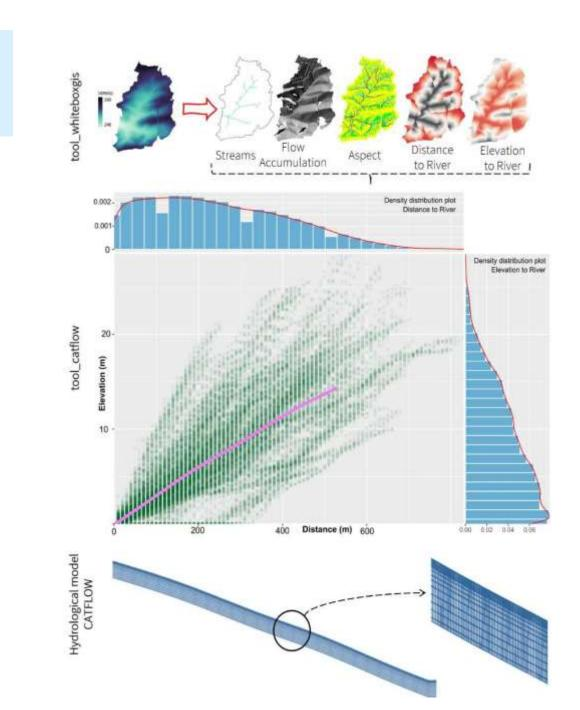
Using **DEM2CAT**, it is possible to reproduce the methodology from Manoj et al. (2024) 2 to extract representative hillslope catenas based on elevation and distance-to-river distributions. This aids in setting up process-based models to characterize flash floods in small headwater catchments.
