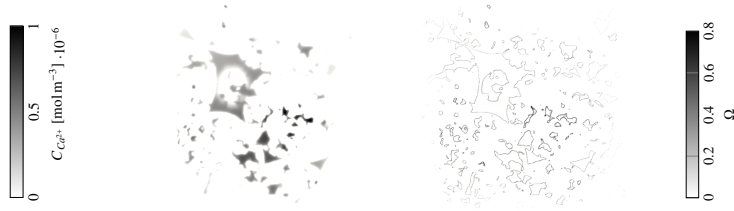
Figure 5.26.: Spatial distribution of calcium cation concentration and saturation product in the realistic 3D geometry by Setup III at the 170 \mu\text{s} in the middle cut plane.
