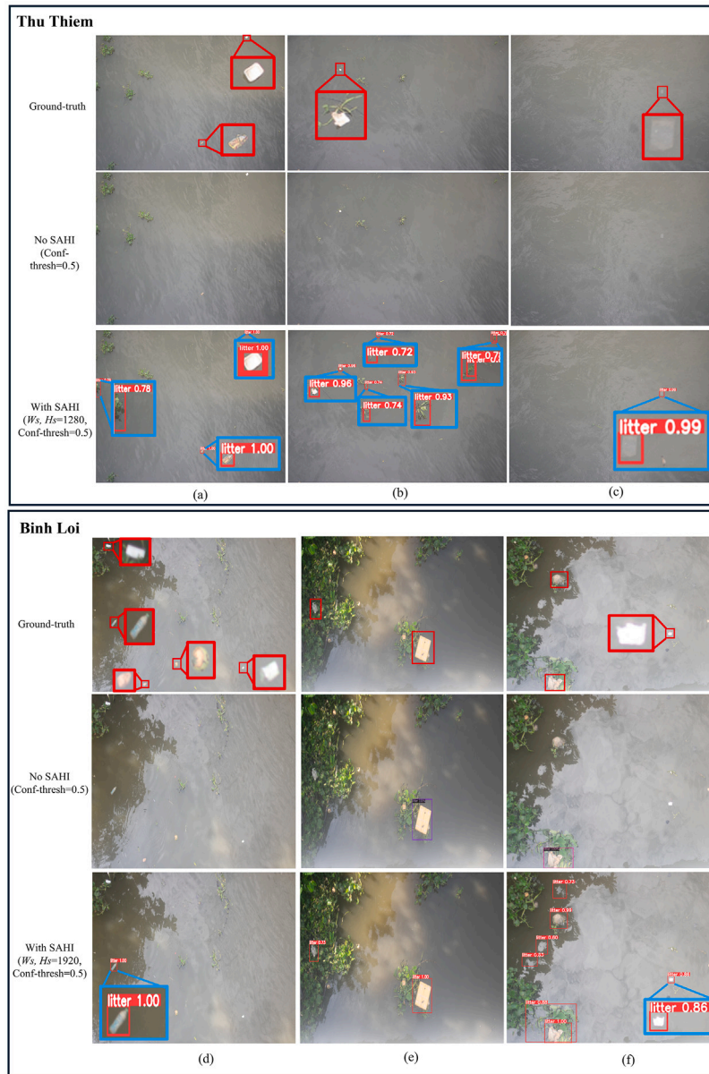
Fig. 7. Examples of predicted bounding boxes for the Faster R-CNN model with and without the SAHI method on the \text{Test}_{\text{Thu Thiem}} ((a)–(c)) and \text{Test}_{\text{Binh Loi}} ((d)–(f)) subsets. We used the SSL method to develop the Faster R-CNN model, that was fine-tuned on the \text{Train}_{100\%} subset. During inference, we set W_s and H_s to 1280 pixel for Thu Thiem case and 1920 for Binh Loi case, with a confidence threshold score of 0.5. Without the SAHI method, the model fails to detect all “small” litter items with area below 1000 \text{cm}^2 in (a)–(f), while correctly detects two “big” items with area above 1000 \text{cm}^2 in (e) and (f). With SAHI, the model correctly detects some “small” items in (a)–(f) as well as two “big” items in (e) and (f). Acronyms used: Confidence threshold (Conf-thresh).
