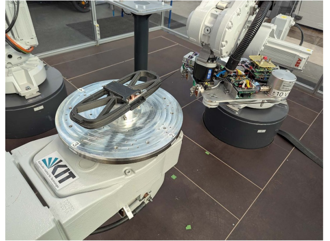
Figure 2. Winding test of the non-planar superellipse coil using the robotic setup.
