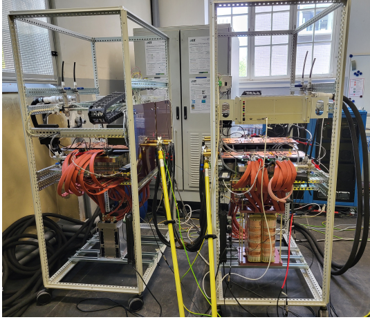
Fig. 3: Two 450 kW DABs configured in a back-to-back (B2B) setup.
