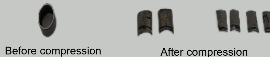
Post-HTO samples - Brittle fracture
