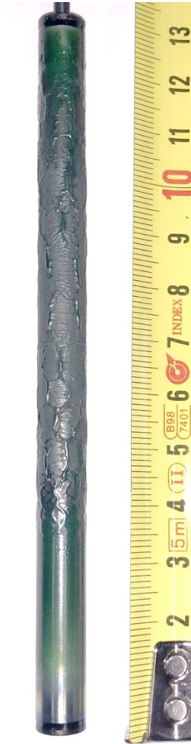
EC1: 8 K/s to T_{\max}=1390\text{ }^{\circ}\text{C} , immediate cooldown
