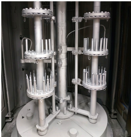
The chamber of the Hauzer Flexicoat 850 coating machine – PVD, FS, ČVUT
