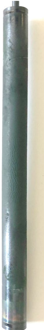
MC-5: 1200 °C during 15 min
