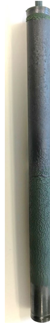
MC-6: 1350 °C during 5 min
