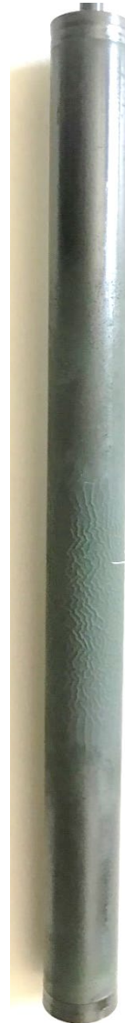
MC-7: 1250 °C during 10 min
