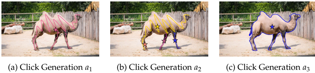
Figure 4.3: Visualization of our click generation strategies. For (a) and (b) a colored star ★ indicates the position of a generated click based on the corresponding colored scribble. For (c) we leverage the mask information directly to compute the central position.
