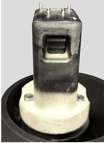
Figure 3. FZJ-RFA2 probe head with Langmuir probes (diameter d = 2 mm, length l = 2 mm) on front face and RFA entrance slits on a side.
