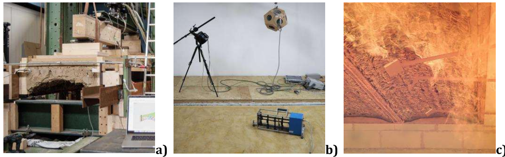
Figure 2. a) Load-bearing test, b) sound test, and c) fire test of the hybrid component ceiling slabs
