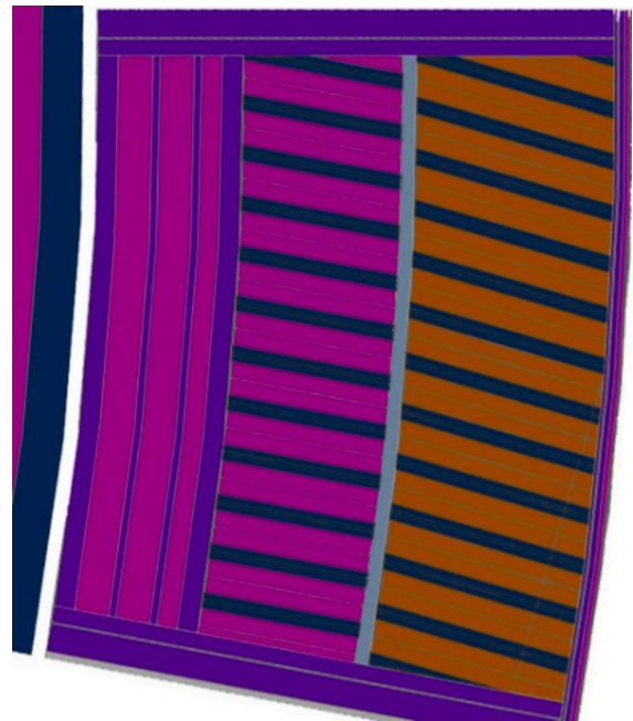
Fig. 6.8. IB equatorial section of the baseline2024 configuration with an additional stiffening steel layer (clear blue) between the front and rear BZ visualized in SuperMC. (For interpretation of the references to colour in this figure legend, the reader is referred to the web version of this article.)
