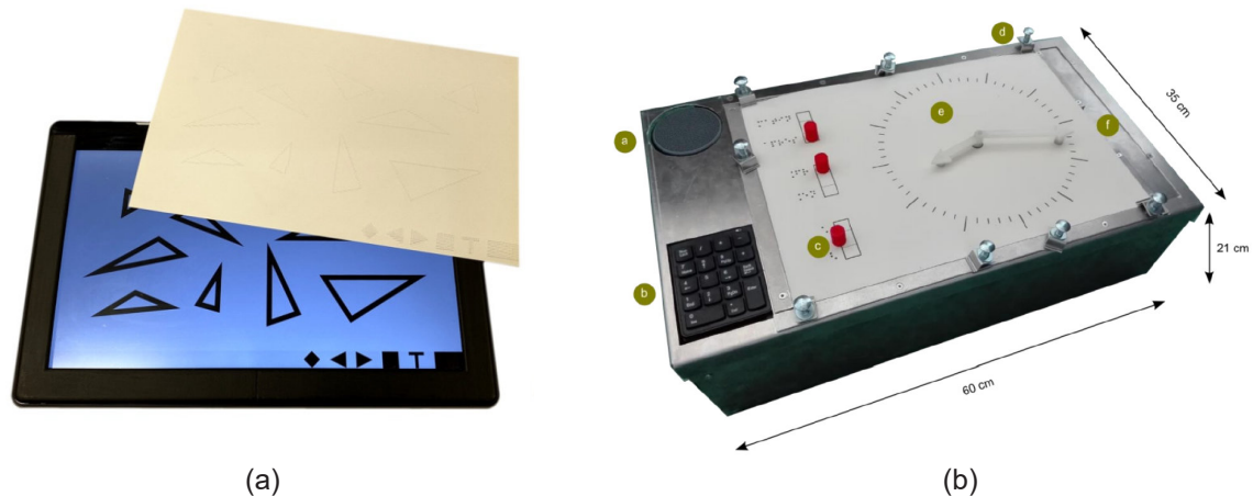
Figure 2.5: Hybrid methods for representing information for users who are BLV: (a) tactile document representation hybrid method by Mackowski et al. [61], (b) FlexiBoard by Raynal et al. [62]
