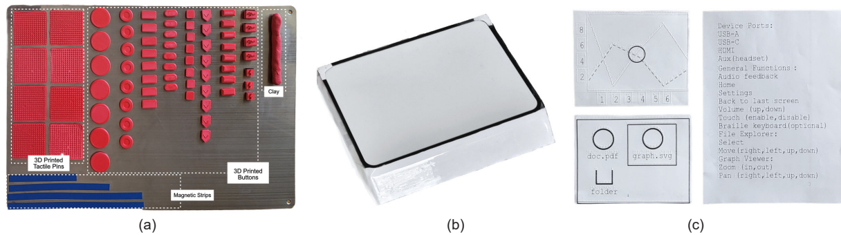
Figure 4.3: Final prototyping toolkit, (a) magnetic board with 3D-printed elements that represent the buttons and control elements of the 2D tactile display, 3D-printed squares that represent the tactile pins, magnetic strips and clay, (b) a box that represents the future device case of a 2D tactile display made from compressed wood with magnetic surfaces on all sides, (c) two embossed papers representing the available software UIs and printed list of base features of the device in Braille.
