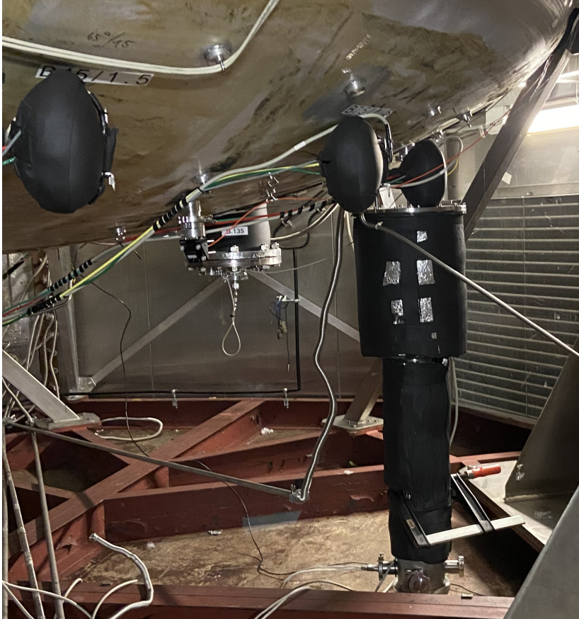
Figure 3.4.: Integration of PHIPS-POL in a vacuum cannister (black cylinder) in the AIDA cloud simulation chamber. The picture was taken during the RICE04 measurement campaign.
