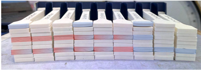
Figure 5.7: Side view of all samples, highlighting extrusion defects on specimens using N01 (non-rectangular outer contour/curvature (blue) and irregularities in the print image (red)), taken from Hauck et al. [4]
