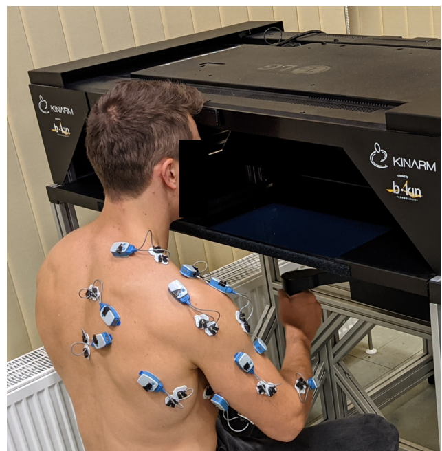
Figure 1. Experimental setup. A participant with EMG electrodes attached sits at the KINARM End-Point Lab (KINARM, Kingston, Canada). EMG, electromyogram.
