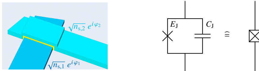
Figure 2.2.: Josephson tunneling junctions (JJs) in this thesis consist of two overlapping aluminum electrodes (dark and light blue), which are separated by a thin insulating aluminum-oxide barrier (yellow), as shown in the left panel (oxide barrier is not to scale). This structure forms a superconductor-insulator-superconductor (S-I-S) junction. The condensate in each electrode is described by its own complex wavefunction \Psi_j = \sqrt{n_{s,j}} e^{i\varphi_j} , coupled through the tunneling of Cooper pairs through the JJ. To account for the geometric capacitance across the tunnel barrier C_J , the junction is represented with a parallel capacitor in the equivalent circuit diagram as shown in the right panel.
