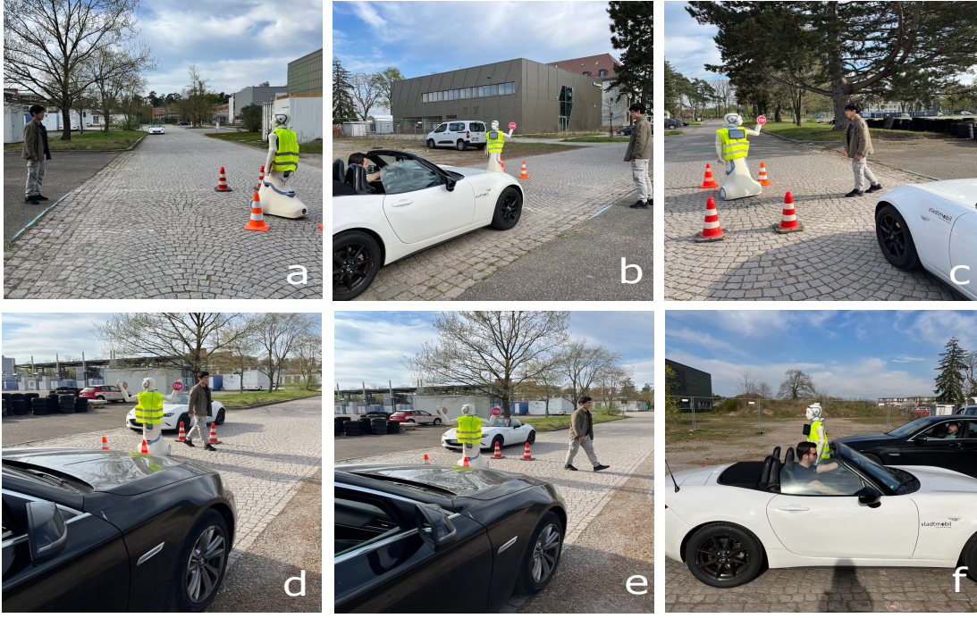
Fig. 1: ARI robot traffic management sequence: (a) detects pedestrian; (b) monitors and stops oncoming vehicles; (c) signals pedestrian to cross; (d) uses rear camera to detect and (e) halt vehicles in the second lane to ensure pedestrian safety; and (f) lets vehicles pass once the pedestrian has completed the crossing.
