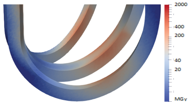
Fig. 7. Distribution of the absorbed insulator dose in the lower section of TFC (10 FPY).
