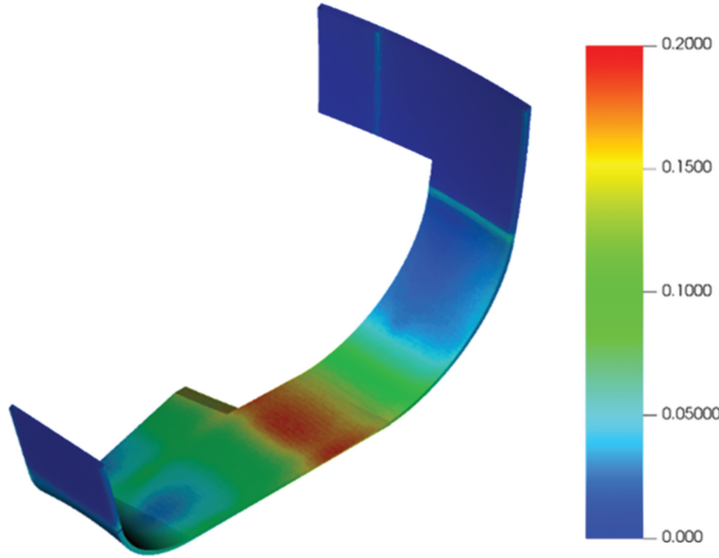
Fig. 8. dpa/FPY distribution at the VV inner shell around the divertor cassette.
