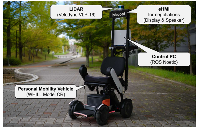
Fig. 1. The APMV with an eHMI can convey driving intentions to pedestrians through voice and visual cues.
