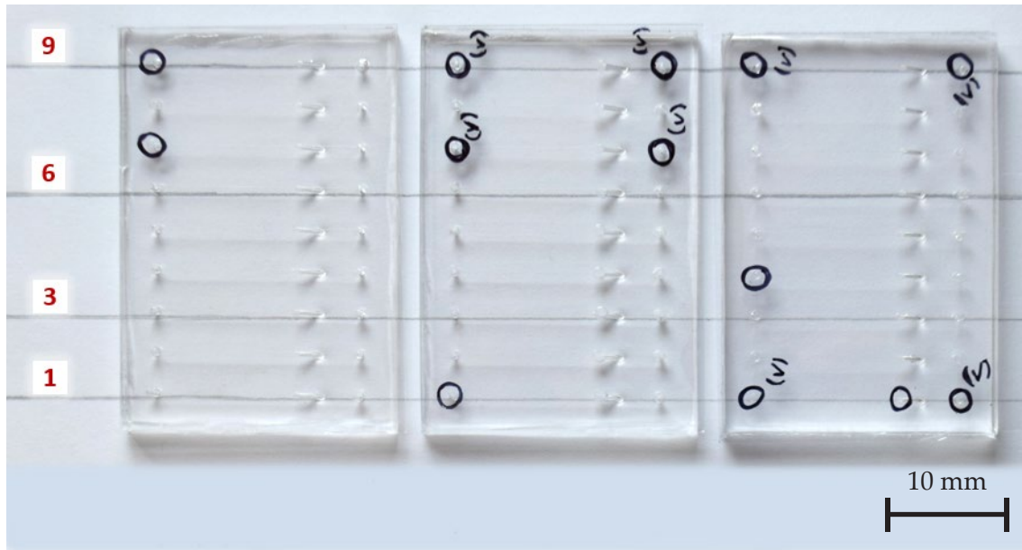
Figure 4.11: Completed 9-channel RCs with mostly functional channels. Circled ports indicate those without flow. Checkmarks denote openings that were initially blocked but could be cleared successfully.
