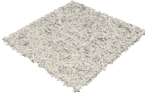
FIGURE 1. Fiber network model of paper at the millimeter scale.
