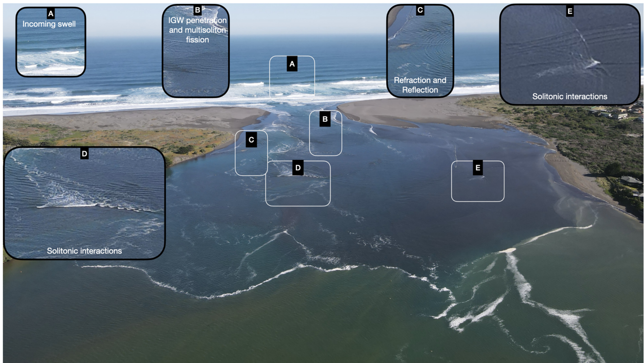
FIG. 14. Snapshot of the wave field during the field experiment where most instances of the conceptual model for the generation of the soliton gas regime at Laguna Cáhuil can be observed. Callouts refer to enlarged inset images. Explanations are provided in the main text.
