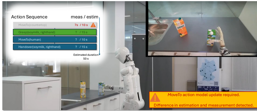
Figure 3.2.: The humanoid robot ARMAR-7 is grasping the milk from the kitchen counter. The grasping action is part of a plan where the robot first moves to the counter, grasps the milk, moves to the human, and finally hands the milk over to the human. The moving action to the counter has already been executed, whereby the estimated duration and the measured duration of the action execution differ significantly.
