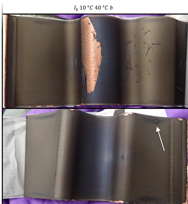
Figure 4.19: Picture of negative electrode sheets of “L 3.4” with the aging condition I_z 10 °C 40 °C b.
