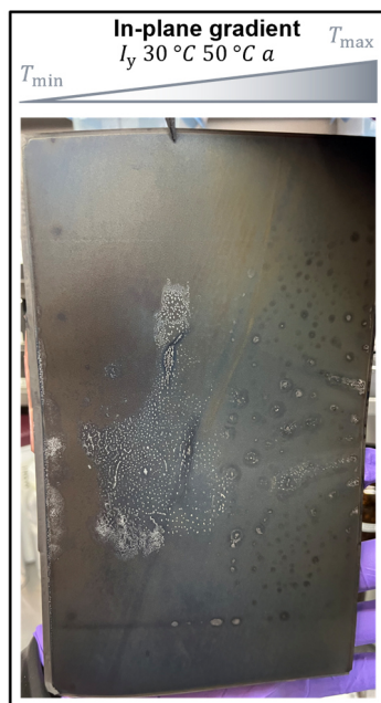
Figure 4.7: Picture of negative electrode sheet of aged “Enertech” I_y 30 °C 50 °C a (Reproduced with permission under the terms of Creative Commons Attribution 4.0 License CC BY.[1] Copyright 2025, The Authors. Energy Technology published by Wiley-VCH GmbH.).
