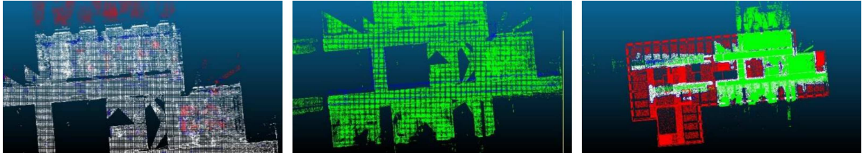
Fig. 6. The technology initiative, 3D points in green colour represent sensor data, 3D points in blue colour are BIM model, and 3D point cloud in red colour show the missing build elements.
