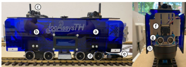
Fig. 2 Scaled demonstrator with (a) Raspberry Pi, (b) Arduino Nano, (c) Marvelmind Beacon, (d) Rotary Encoder, (e) Strain gauge, (f) RGB camera, (g) Ultrasonic sensor, (h) LiDAR [19]
