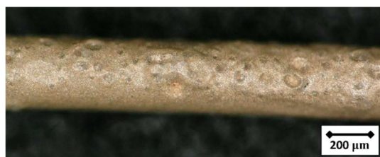
Figure 62 Examples for occasionally occurring defects during the wire coating process. Typically, a combination of air inclusions and craters caused by inhomogeneously evaporating solvent.
