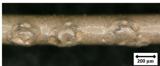
Figure 62 Examples for occasionally occurring defects during the wire coating process. Typically, a combination of air inclusions and craters caused by inhomogeneously evaporating solvent.
