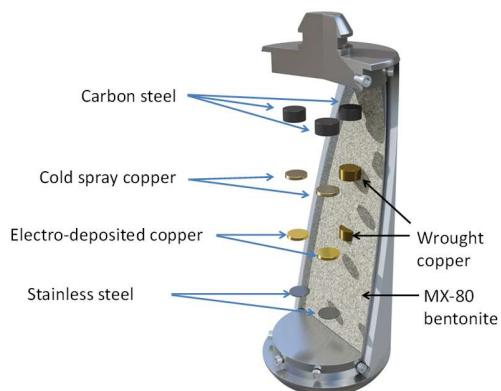
Figure 1. Layout of metal coupons in each module.
