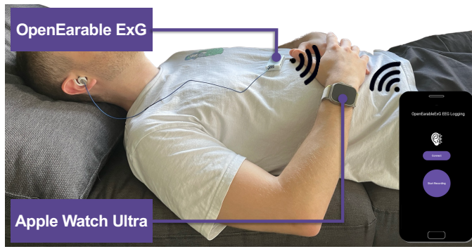
Figure 2: Overview of the sleep experiment. A participant is wearing the OpenEarable ExG with in-ear electrodes, resting on his chest, and an Apple Watch Ultra. OpenEarable ExG streams data to a corresponding app via Bluetooth.
