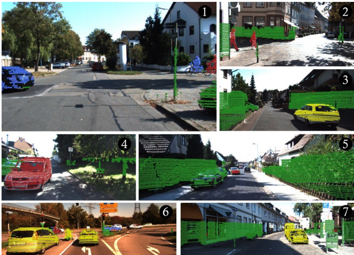
Figure 7.7.: Supervised Model Failures: These exemplary images show model failures of the supervised stream, which can be detected due to contradicting outputs of the self-supervised model. Scenes from the KITTI dataset [146]. Reprinted from [BOG 20].
