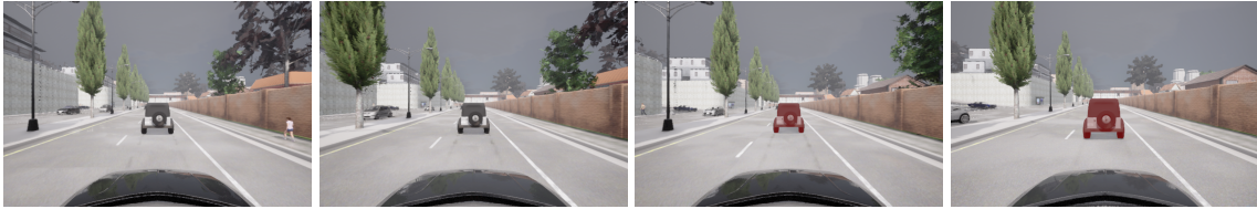
Figure 4.8.: Temporal anomalies: This scenario shows the implemented type of temporal anomalies. The first two images show the regular vehicle following mode. The last two images show the active braking maneuver with overlaid ground truth in red. Reprinted from [BOG 6].
