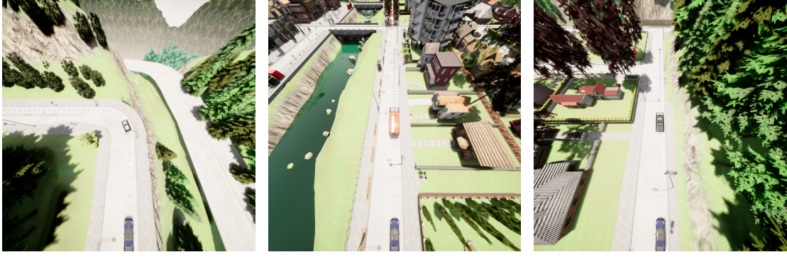
Figure 6.4.: Benchmark: Exemplary scenarios with different object-level anomalies blocking the lane. The dotted lines in front of the ego vehicle represent the reference trajectories towards the goal. Reprinted from [STU 6].
