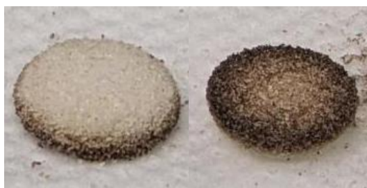
Figure 7-21 Residual crucible material at the \sim 40 \text{ nm}\cdot\text{min}^{-1} equivalent sublimation rate. Original (raw) source material was taken from the same batch of FAI as Figure 7-14 . Reproduced from Wiley-VCH GmbH ©2025 with permission. 504
