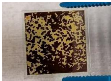
Figure S6-5 Camera image of perovskite film grown on solution-processed bulk Me-4PACz. This filter corresponds to the highest performance stoichiometry. The two distinct colors indicates two different perovskites form on the same sample, highlighting surface inhomogeneity. Figure reproduced from Elsevier Inc ©2024 with permission. 221
