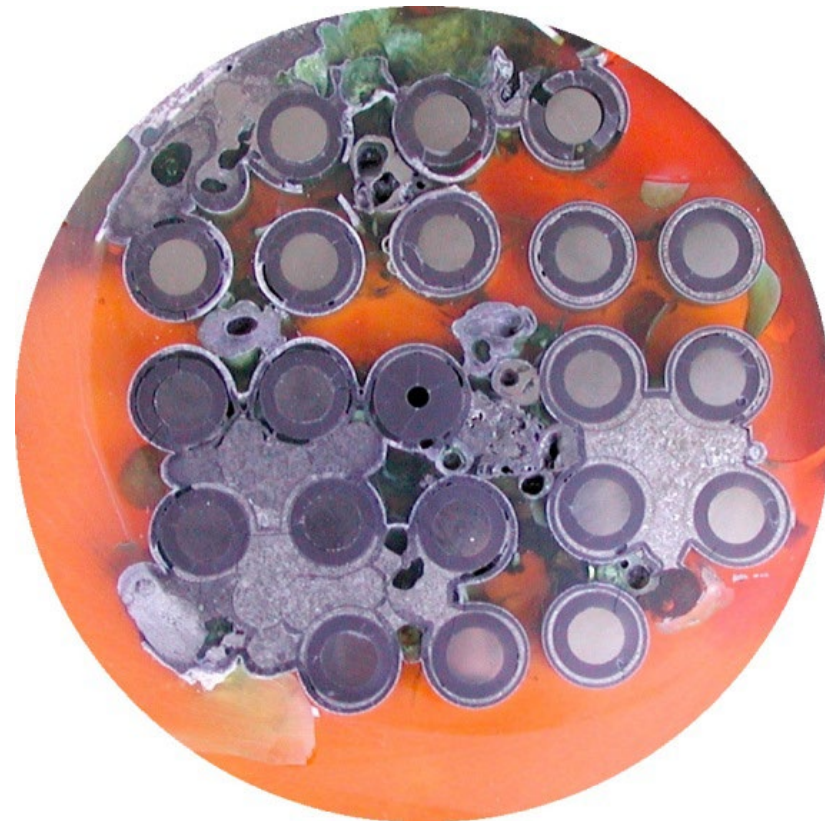
PWR QUENCH-11 ( T_{\text{pct}} \approx 2100 \text{ K} ), elevation 837 mm: formation of large molten pools below the bundle hot region
