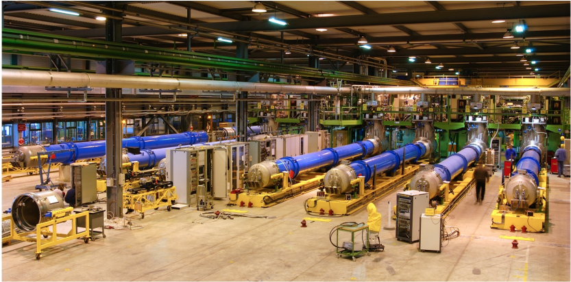
Figure 2.4: Cryogenic, horizontal test benches with different LHC magnets in different measurement stages. From “LHC dipole testing facility completed” by Brice (2004).
