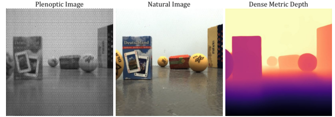
Fig. 1: Left : Plenoptic image from a light field camera, displaying the microlens pattern (see detail in Fig. 2). Center : Corresponding natural image, synthesized from the central viewpoint of the plenoptic camera. Right : Our single-shot metric depth map, at the true scale of the scene.
