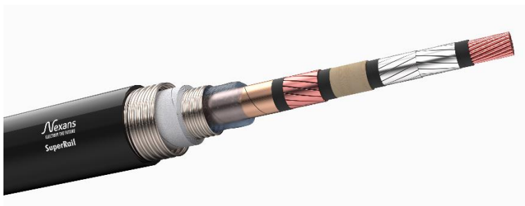
Figure 2. SuperRail 3.5 kA / 1.5 kVDC Superconducting cable (HTS) developed by Nexans for the French Railways (SNCF) to be pulled in existing 100 mm diameter pipe
