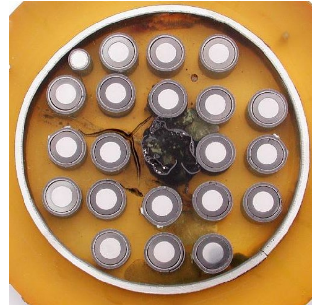
QUENCH-07 bundle: thick oxide layers after oxidation in steam
