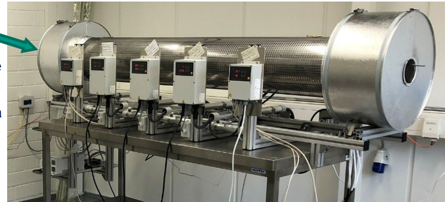
HOKI oven with axial temperature profile: T \approx 450 \text{ }^\circ\text{C} along the length of \approx 1250 \text{ mm}
