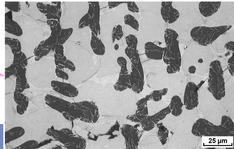
ceramic precipitates in the cladding-pellet gap : 35% area acc. to image analysis
