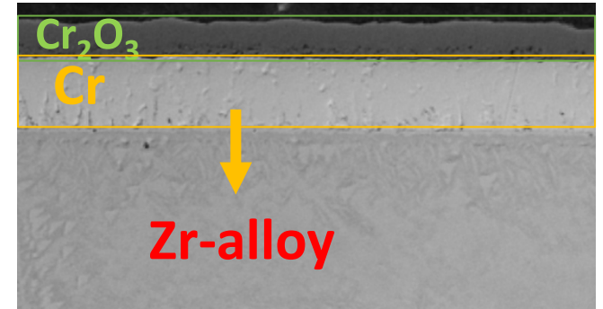
Zr-alloy with protective coating - 1200°C/30 min
