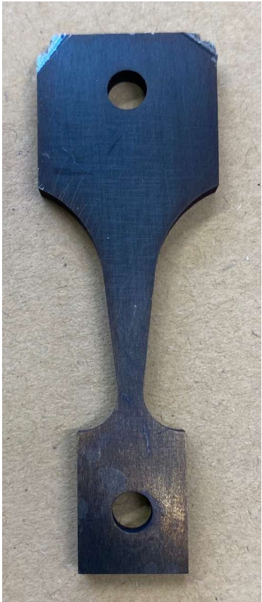
Tensile samples with stress/strain gradient
