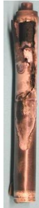
Post-test appearance and axial cross-section of a specimen after 30 min isothermal test at 1470 °C
