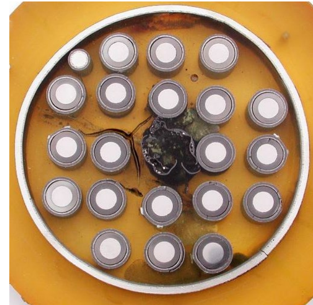
QUENCH-07 bundle: thick oxide layers after oxidation in steam
