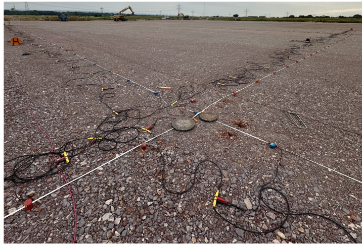
Figure 3.2: Field view at the profile intersection near K0. White tapes mark the two survey lines; geophones are spaced at 1 m with visible cabling. This photo documents the layout and surface conditions during acquisition. Source: Rasho (2025).
