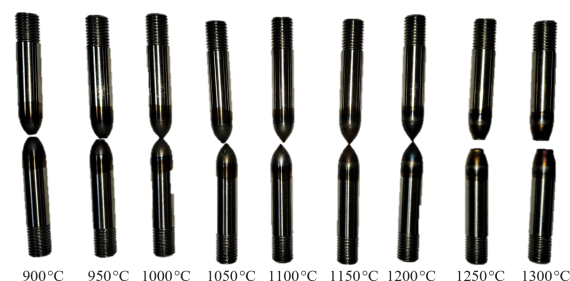
Figure 5. Image of the 45SiCrV9Ni hot tensile test samples after the experiments, depicting their fracture behavior depending on the test temperature indicated below each sample.
