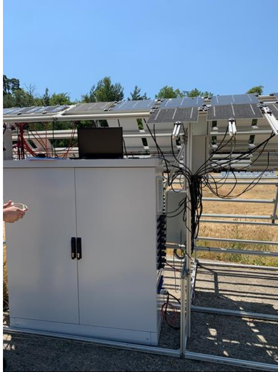
Figure A6.1: Cabinet with with electrical components to protect them from environmental factors.
