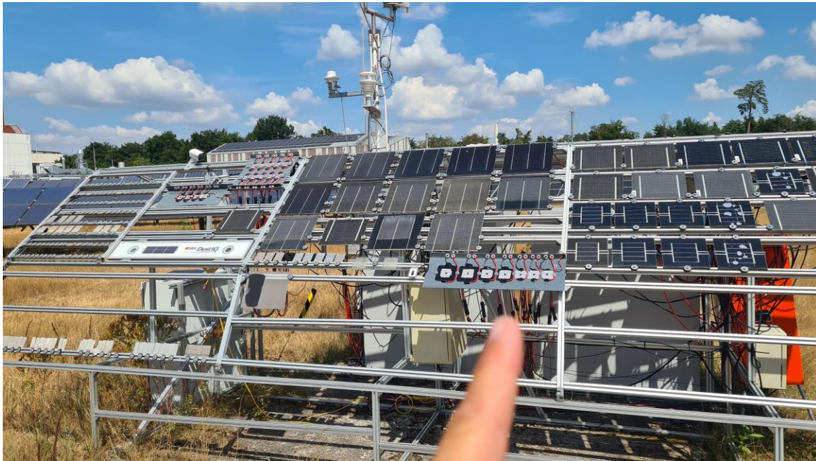
Figure A6.5: Bosch profile structure for fastening solar cells for measurement in the outdoor condition. A camera monitors the samples for obstruction.
