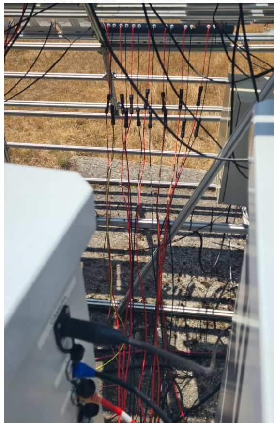
Figure A6.4: Waterproof MC4 connectors for connecting solar cells with the electrical connectors. The connection of irradiance sensor (black) and LAN (blue/red) to the cabinet is also waterproof.
