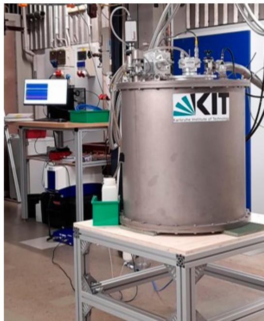
Figure 5. Picture of the magnet on a stand in the front and the NMR control units in the back.
