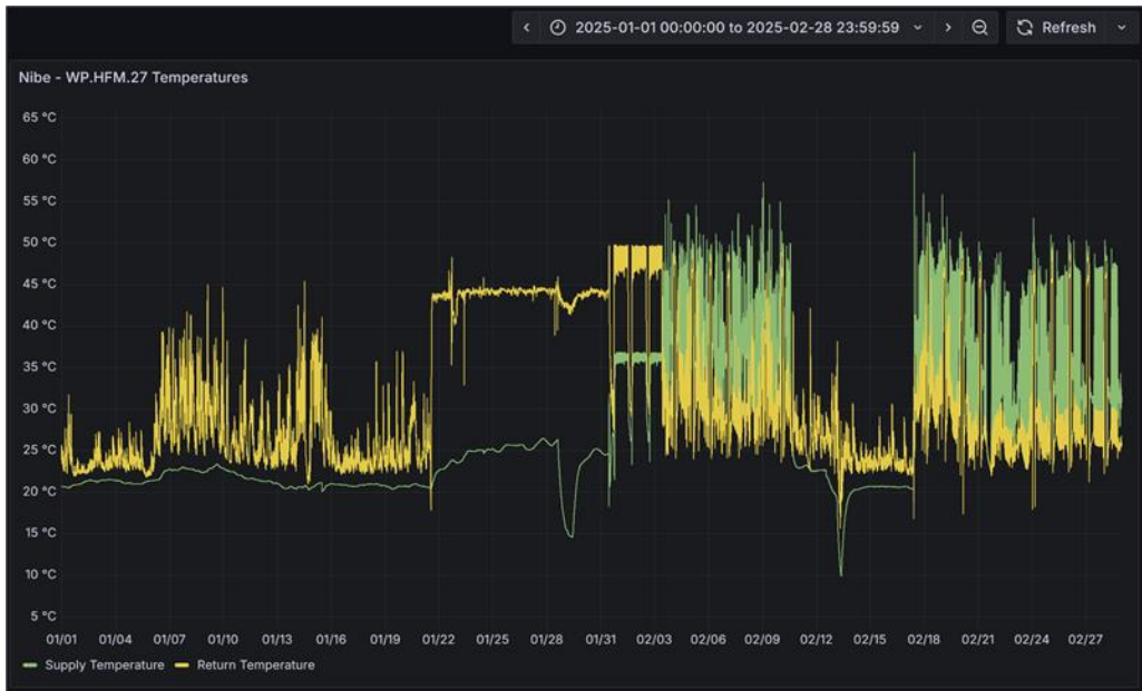
Figure 4.5: An illustrative example of the supply and return temperature of the experimental GSHP from January 2025 to February 2025 on Grafana
