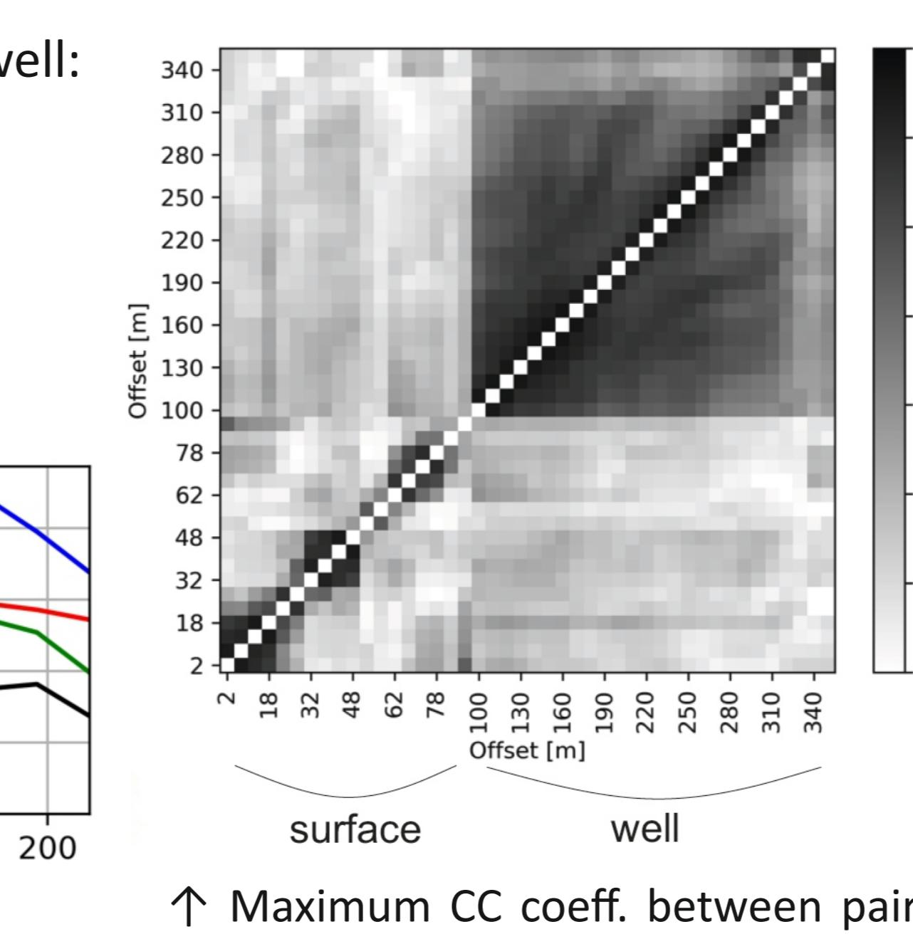
↑ Maximum CC coeff. between pair of channels, mixing surface (BP filtered) and well (BP+fk) sections
