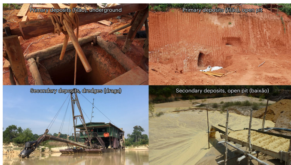
Fig. 1 | The four main mining types of ASGM in the Tapajós. Photographs show (clockwise from top left) underground mining of primary deposits ( filão ), open pit mining of primary deposits ( filão ), open pit mining ( baixão ) of secondary deposits and dredge mining ( draga ) of secondary deposits.
